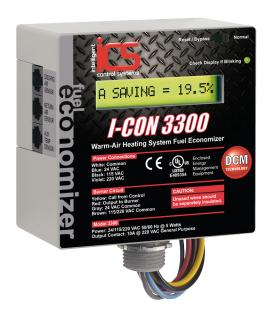
*i-CON* is a microprocessor-based, fuel-saving control for warm air heatings systems. *i-CON* 3300 reduces burner run time, eliminating harmful heat exchanger over heating and reducees fuel consumption, when installed on any new or existing warm air furnace or combination RTU. *i-CON* 3300 uses intelligent Dynamic Cycle Management (DCM) technology to save energy by adjusting the burner run pattern to manage the discharge air temperature based on the system's "heating load."
